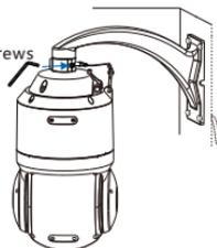
3. Twist off the 2 positioning screws on the upper housing and open the upper housing. Hang the safety hook on the housing on the convex screw on the housing.
